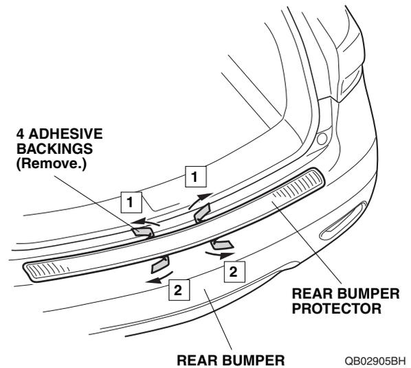
13. Using a rubber roller, apply firm pressure to the rear bumper protector, especially at the ends, as shown.
