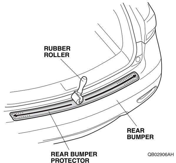
14. Secure the rear bumper protector to the rear bumper with the four clip holders.
