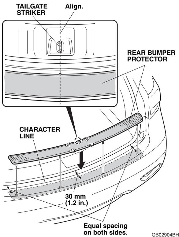
12. While applying light pressure against the rear bumper protector, carefully remove the adhesive backings in the order as shown.
